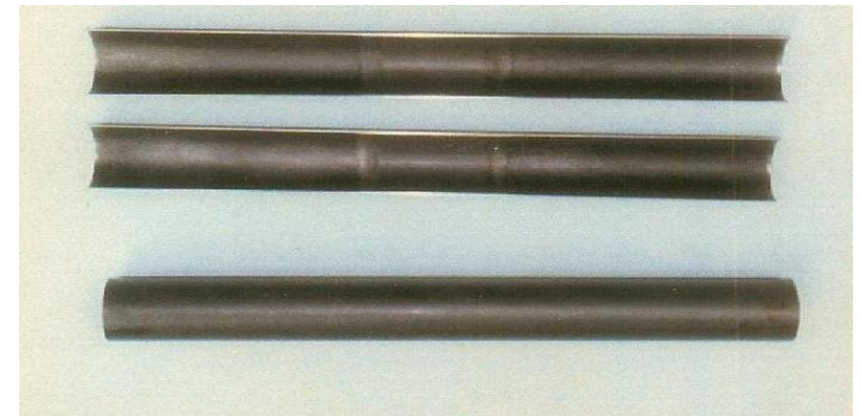
CHEMICAL MILLING OF SPAR TUBE (1/6 th MODEL)
