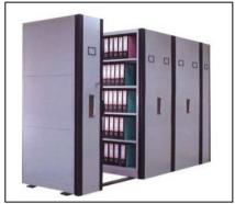
It consists of storage units (Depth 450 to 470 mm, width 850 to 950 mm and height 1900mm to 2000 mm) – fixed / movable – bolted to Undercarriage which rolls onto the channels, which, are firmly embedded to the ground. Rigid Knock Down construction made out of 0.8 thick CRCA Steel. Each body block (SS/SL/TM) building consists of 1 Main unit & then Add-on units. Each unit has 5 loading levels formed by 4 no's adjustable shelves.
