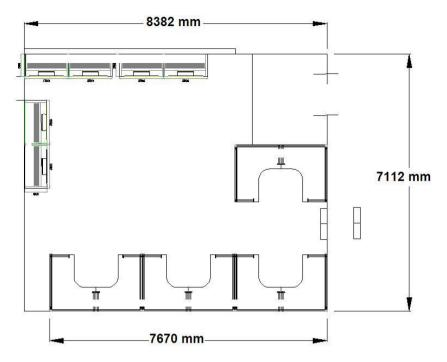
Fig. 1 Layout for Linear and L shaped computer work station tables
