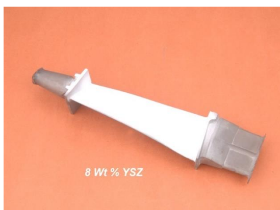
Plasma sprayed YSZ coating on a gas-turbine blade
