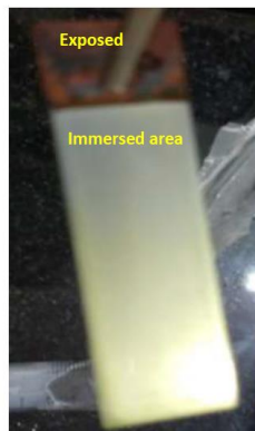
C1018 IN ACID SOLUTION DOPED WITH NAL INHIBITOR - > 6 MONTHS
